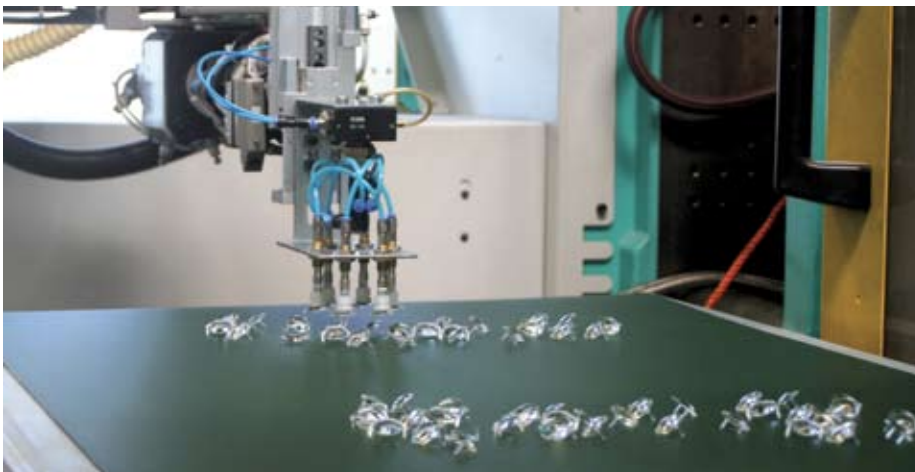
Automatic machine producing reflector lamp lenses
